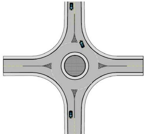
Roundabouts require the rights-of-way, similar to a traditional intersection. Parking is prohibited on the approaches and around a roundabout. Pedestrian and bicycle crossings are generally not permitted within the roundabout. Therefore, this traffic calming measure should not be used on streets with high pedestrian and bicycle volumes.
