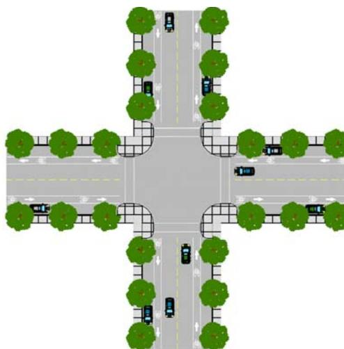
Neckdowns and bump outs can also be used at mid-block locations to provide areas for benches and plantings, which improve the aesthetics of the neighborhood. Vertical elements, such as light poles, trashcans, benches and trees, can also be used to draw attention to the constriction of the road and provide a visual cue to the motorist.
