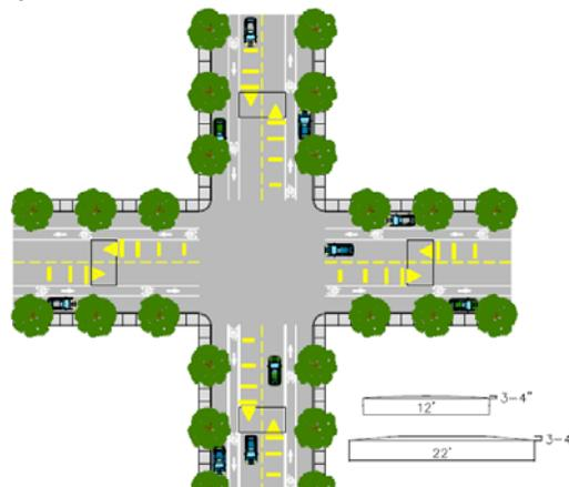
Figure 4.7-1 Speed Humps
