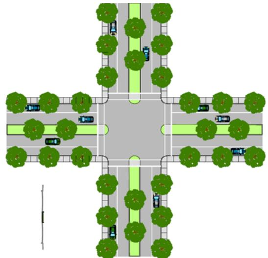
Median islands are appropriate for local, collector and arterial streets and may be used on high-volume roads with posted speed limits up to 40 MPH. Median islands should be 6 to 8 feet wide and should be at least 12 to 20 feet in length. Access across the raised median should be provided in the design to accommodate pedestrians and bicyclists. Raised medians will restrict access to driveways to/from one direction of travel.
